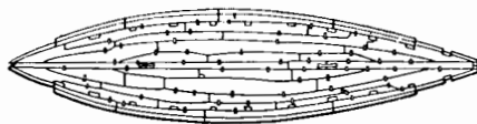
EGYPTIAN BOAT OF WOOD, 2000 B.C. DOVETAILS OF HULL CONSTRUCTION, SEEN FROM ABOVE
